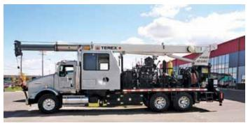
Terex B.T. 3063 rated to 15 tons with 19m of stick, equipped with Cranesmart
