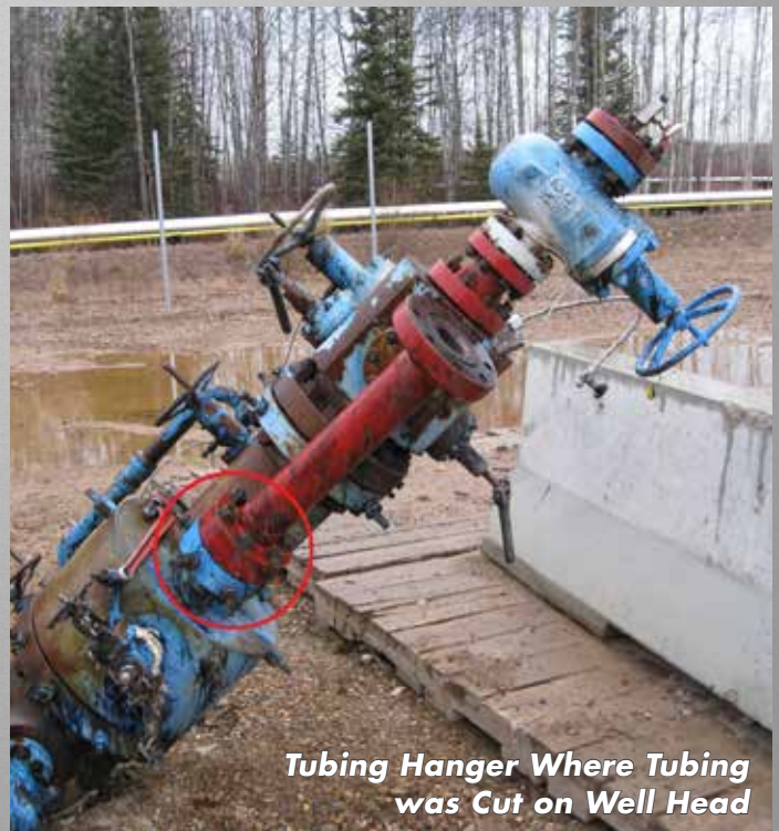
Cut Tubing Below Hanger
