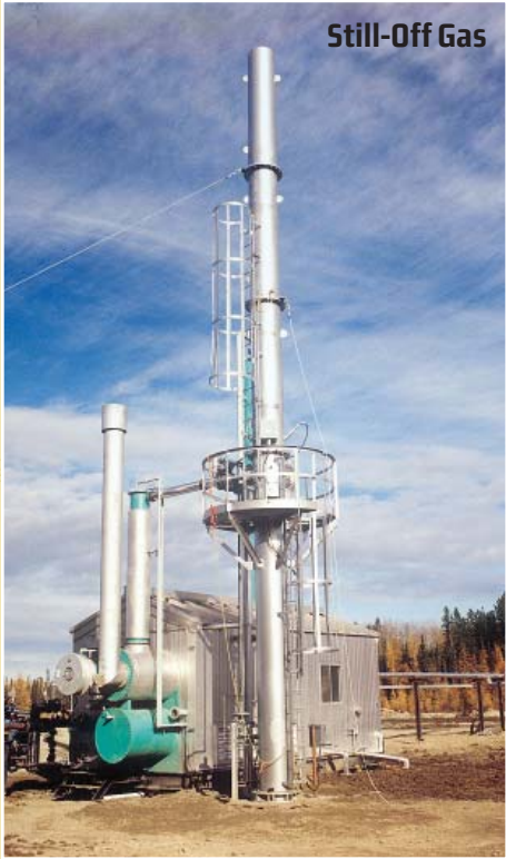
Still-Off Gas Tornado designers pioneered the industry's first dehydrator still-off gas incinerator (SOGI) over 20 years ago. The same unit still operates in the field today.
